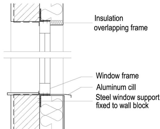
Figure 1. Window installation with minimised thermal bridge
